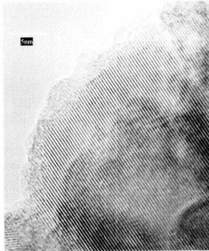
Fig. 3.4 TEM image of a titanium dioxide pigment particle with an inorganic surface treatment consisting of SiO 2 and Al 2 O 3 (courtesy of T. A. Egerton)
