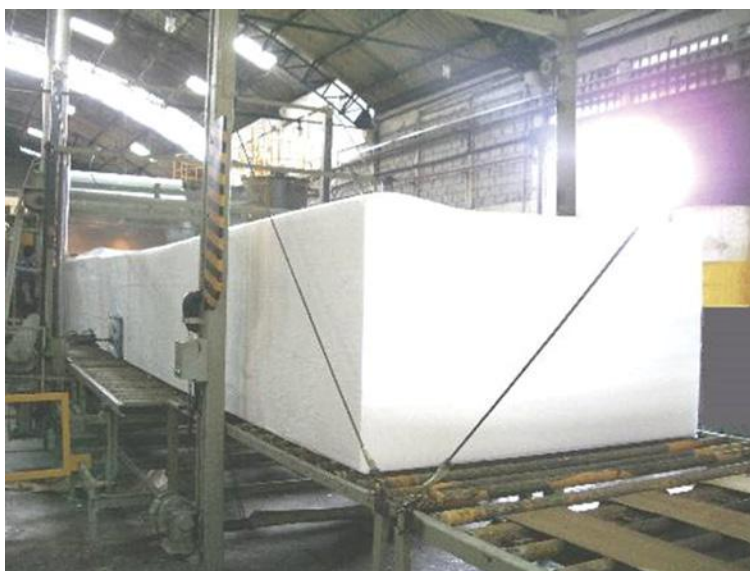
FIGURE 6.1 Slab foam process. The image does not show the feed tanks, ventilation, or substantial amount of electronic controls involved. Reprinted with permission from Ref. [3]. © John Wiley & Sons, Inc.
