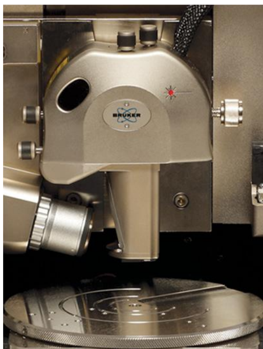
FIGURE 5.7 Simplified illustration showing sample and signal detection controls for a tapping mode atomic force microscope and the appearance of a working instrument. Images courtesy of Bruker Nano-Surface.
