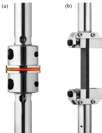
FIGURE 5.26 DMA fixtures: (a) parallel plate fixture for measurement of thin solid samples in shear or reacting liquids and (b) torsion fixture for measurement of solid sample viscoelastic properties. Fixtures are carefully engineered and machined to provide minimal compliance and minimum mass. Images courtesy of TA Instruments. © 2013.
