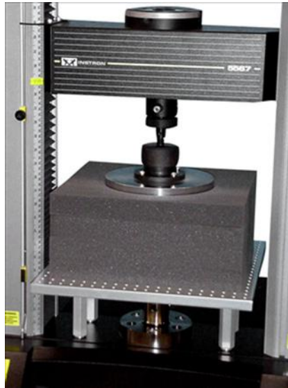
FIGURE 7.4 Test fixture and sample geometry for testing flexible foam indentation force deflection (IFD), a common test for furniture applications. Image courtesy of Instron Corporation.
