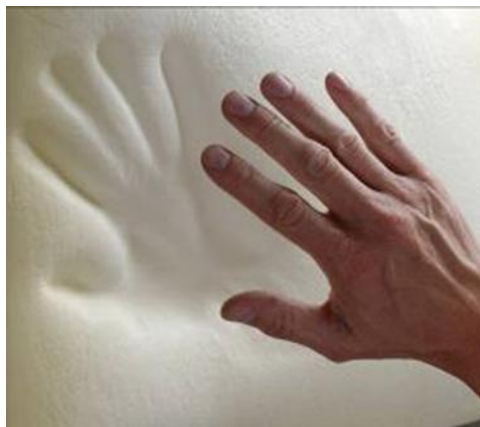
FIGURE 7.7 Illustration of the delayed recovery response of a polyurethane viscoelastic foam. Image courtesy of The Dow Chemical Company.
