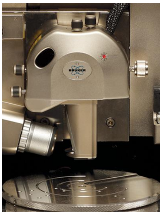
FIGURE 5.7 Simplified illustration showing sample and signal detection controls for a tapping mode atomic force microscope and the appearance of a working instrument. Images courtesy of Bruker Nano-Surface. (See insert for color representation of the figure.)
