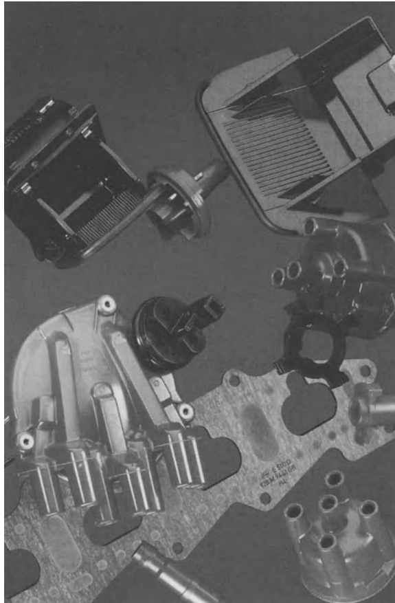
Fig. 6.47. Applications of phenolic molding compounds in the automotive industry (ignition, ashtrays, insulating flanges, etc.)
