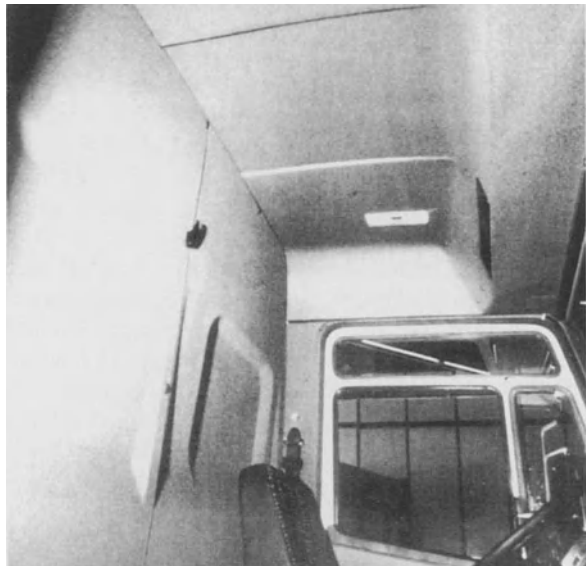
Fig. 6.22. Roof and wall panels of textile felt moldings for a truck interior (source: J. Borgers GmbH & Co. KG, Bocholt)
