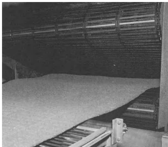
Fig. 6.18. Textile felt fabrication – semifinished goods outlet (source: J. Borgers GmbH & Co. KG, Bocholt)
