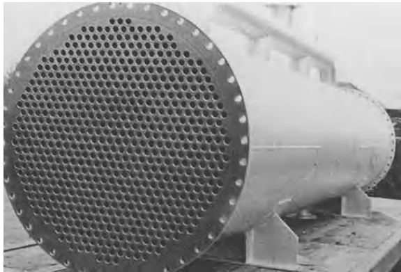
Fig. 6.174. Condenser with interior tubes protected against corrosion with special-purpose, phenolic-based combination binders
