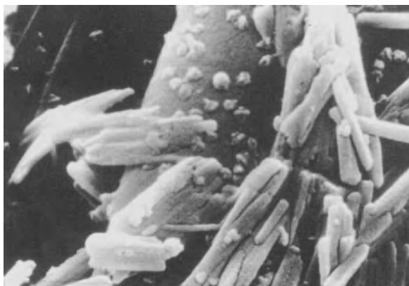
Fig. 6.202. Scanning electron micrograph of carbon from pyrolysis of a novolak-hmta resin in an oxygen-containing atmosphere, slow heating rate
