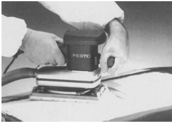
Fig. 6.150. Automotive repair – sanding of filler, strips with holes on electric orbital sander (photo: Hermes Schleifmittel GmbH & Co, Hamburg)
