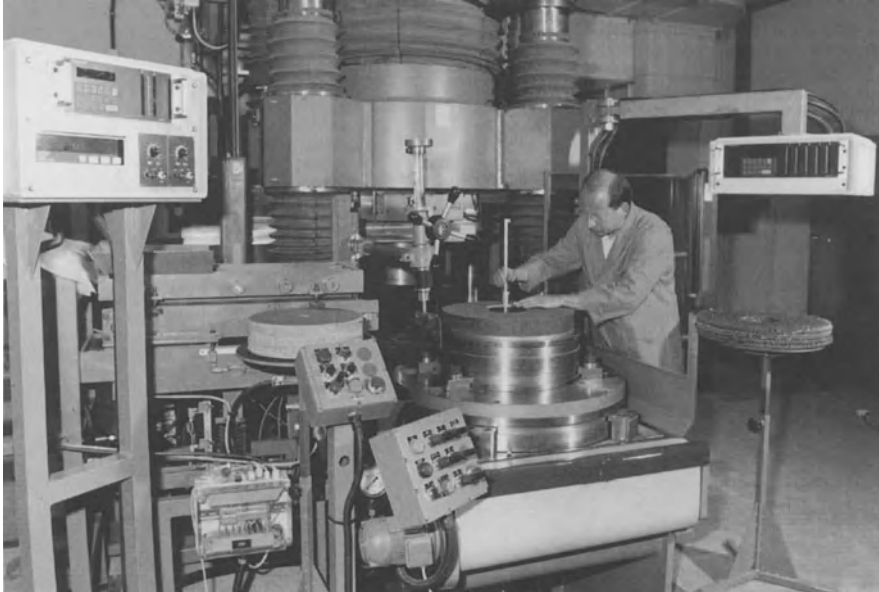
Fig. 6.129. Production of grinding wheels on hydraulic presses (photo: Krebs & Riedel, Bad Karlshafen, Germany)
