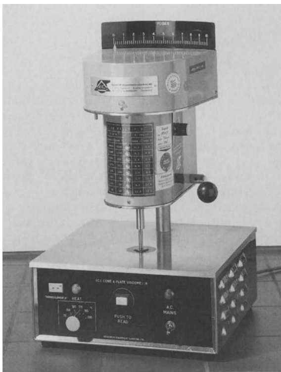
Fig. 7.4. ICI Cone-and-plate viscometer for rapid viscosity determination (photo: Bakelite AG, Iserlohn, Germany)
