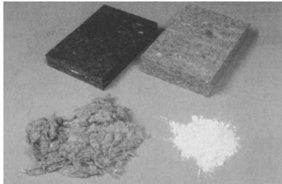
Fig. 6.17. Powder resin, shredded fiber, sheet goods – raw materials and final textile felt product (source: J. Borgers GmbH & Co. KG, Bocholt)
