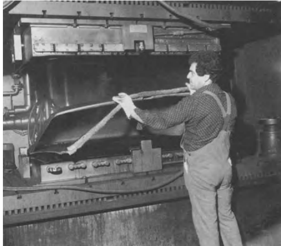
Fig. 6.19. Stripping of textile felt compression molding (source: J. Borgers GmbH & Co. KG, Bocholt)
