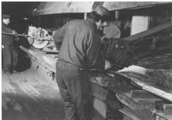
Fig. 6.135. Swing frame grinder for working steel (photo: Tyrolit Schleifmittelwerke Swarovski K.G., Schwaz, Austria)
