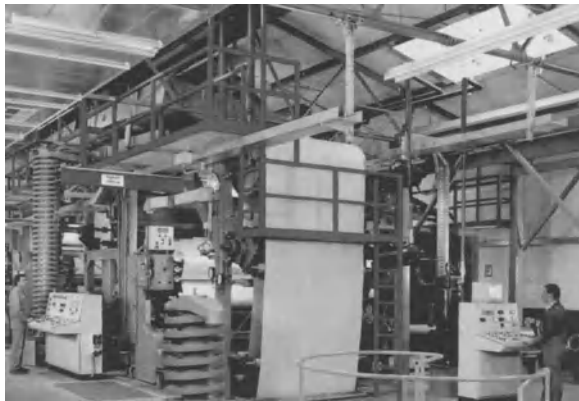
Fig. 6.142. Glue spreader for production of coated adhesives (photo: Klingspor Co., Haiger Burbach)
