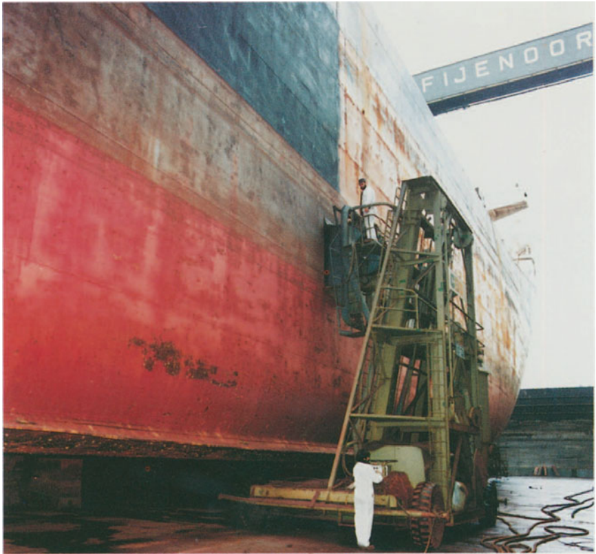
Plate 3. Hydro-blasting of a ship's hull.
