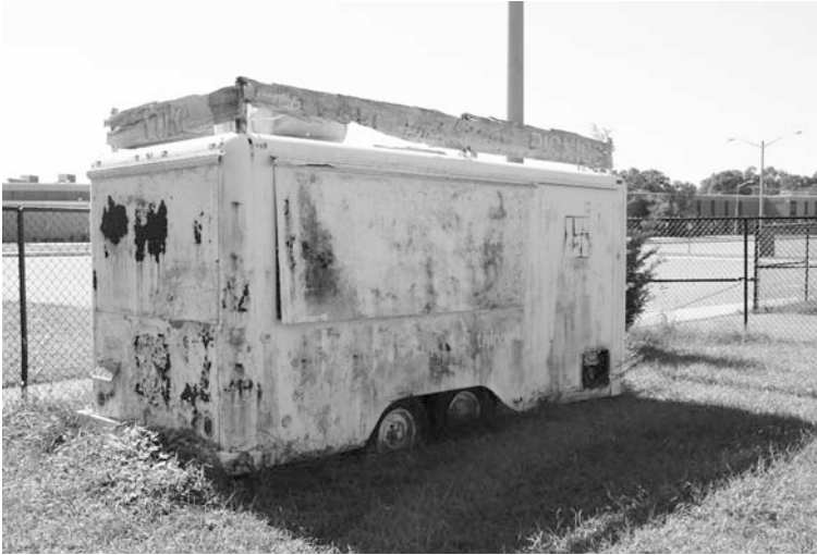
Fig. 13.1 An example of a paint failure leading to corrosion of the underlying substrate
