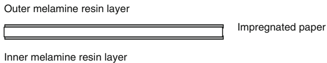
Figure 15 General structure of melamine papers.
