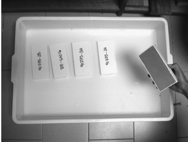
Figure 8 Permeability to liquid water according to EN 927-5 (picture from CATAS spa).
