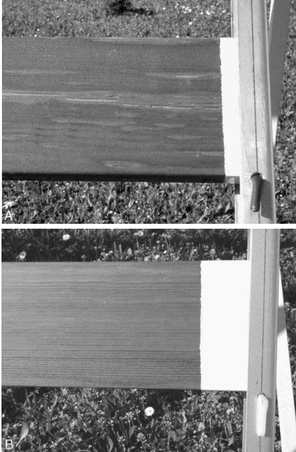
Figure 7 Two different coatings after 1-year exposure according to EN 927-3 (picture from CATAS spa).
