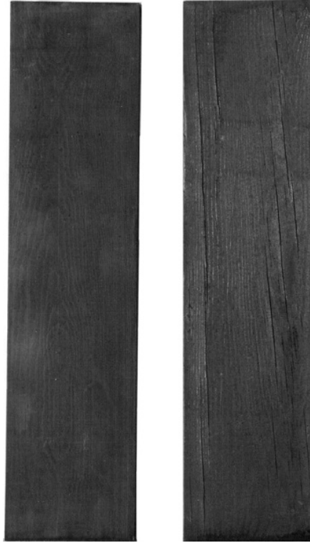
Figure 2 Test panels exposed outdoors (12 months).
