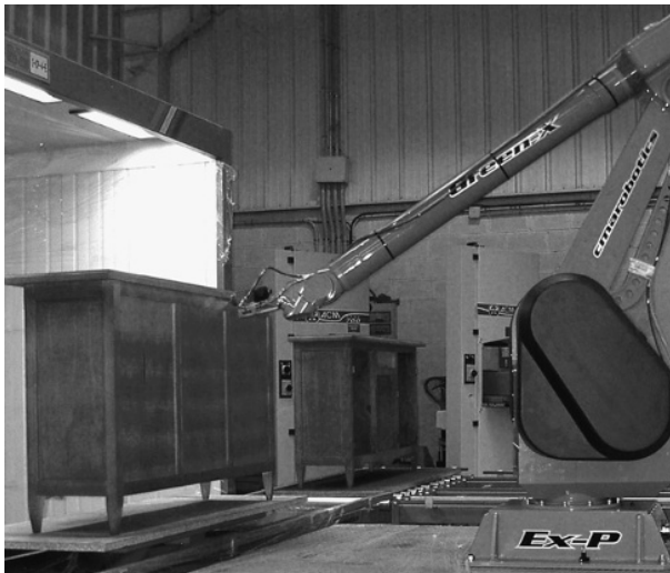
Figure 13 Spray robotic application (courtesy: CMA Robotics spa).
