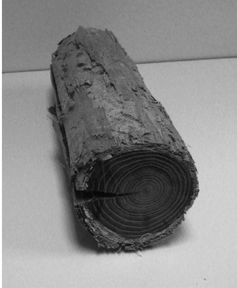
Figure 9 Insect attack on a piece of wood. Sapwood is almost completely destroyed whilst there is no evidence of attack on heartwood.
