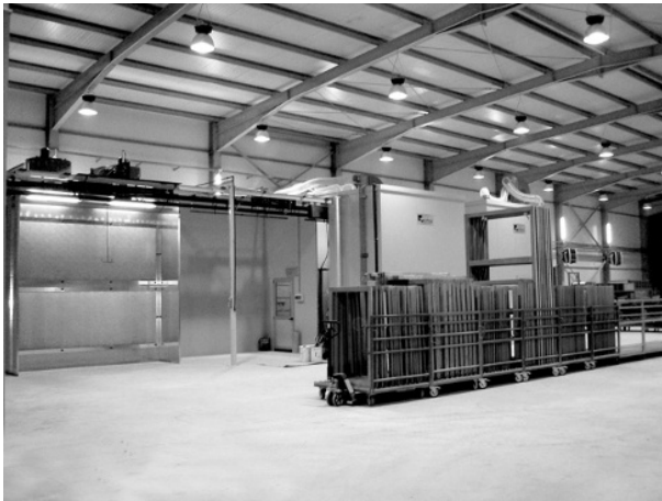
Figure 2 Assembled window frames before the coating process (courtesy: Vertek Group srl).
