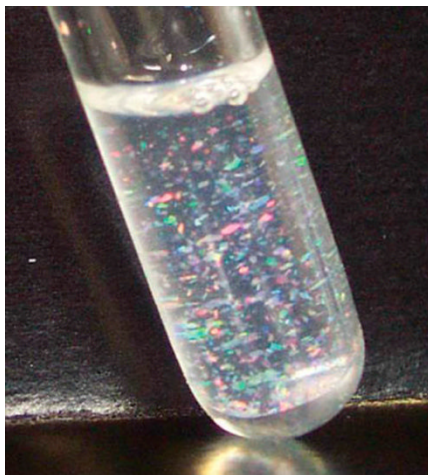
FIG. 9.25 Crystal flakes as effect pigments in a transparent coating. The diameter of the tube is 5 mm. Reproduced from the permission of Ref. 86. © 2004 Wiley.
