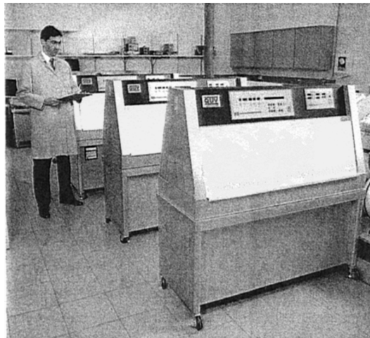
FIGURE 16.2 Accelerated cool white fluorescent testing is fast and easy in the QUV accelerated weathering tester.
