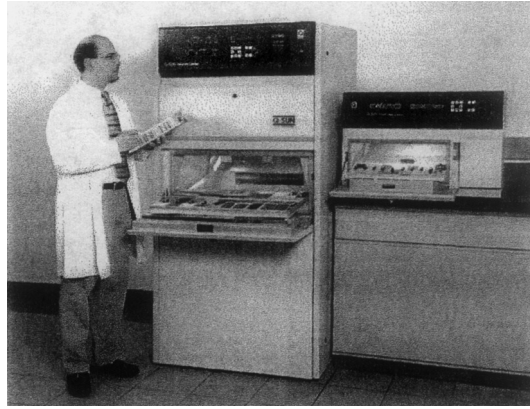
FIGURE 16.3 The Q-Sun Xenon Arc Test Chamber is ideal for subjecting printing inks and substrates to full-spectrum sunlight.
