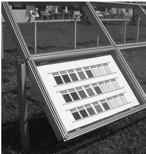
FIGURE 118.3 Ink specimens were placed in ASTM G24 glass-covered exposure racks in Florida and Arizona benchmark locations.
