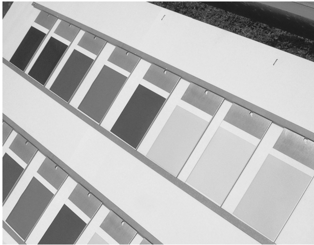
FIGURE 118.2 GATF technical staff selected eight representative lithographic ink colors printed on a standard substrate for fade resistance testing.
