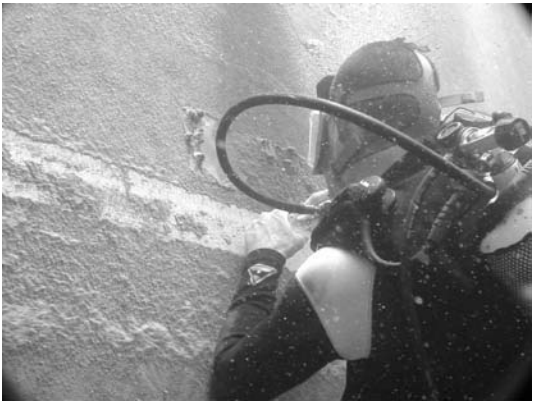
4.12 Example of algal hull fouling on ship's hull.
