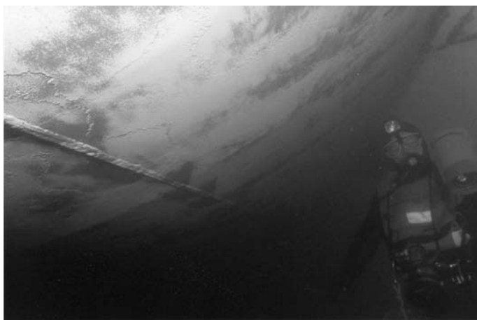
16.5 Picture of a perfectly clean hull during an underwater inspection showing clear signs of polishing. The darker areas (top left-hand side) correspond to the last micrometers of an antifouling layer containing red inert pigments and which has nearly polished-through. Those areas where the red topcoat has been completely exhausted unveil the presence of a white \text{TiO}_2 -containing antifouling undercoat (the leached layer of such paints is completely white). It is interesting to remark that the red topcoat leftovers are found in overlapped areas during paint application (higher initial film thickness).
