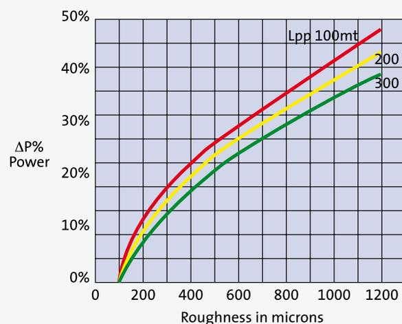
The Graph shows the effect of hull roughness on the percentage increase in Power to maintain speed for several vessel lengths. It shows for instance that smaller vessels are more effected by increasing hull roughness.
