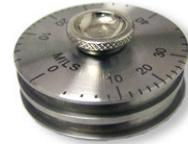
Various measurement ranges are available from 0 to 25 $\mu$ m to 0 to 3000 $\mu$ m (0 to 1mil - 0 to 40mils) are available
